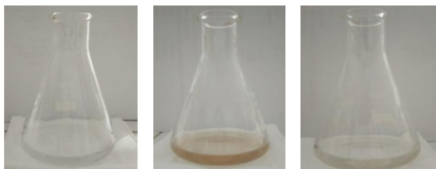
Figure 3. The alteration of vitamin C after reacted with \text{KMnO}_4
