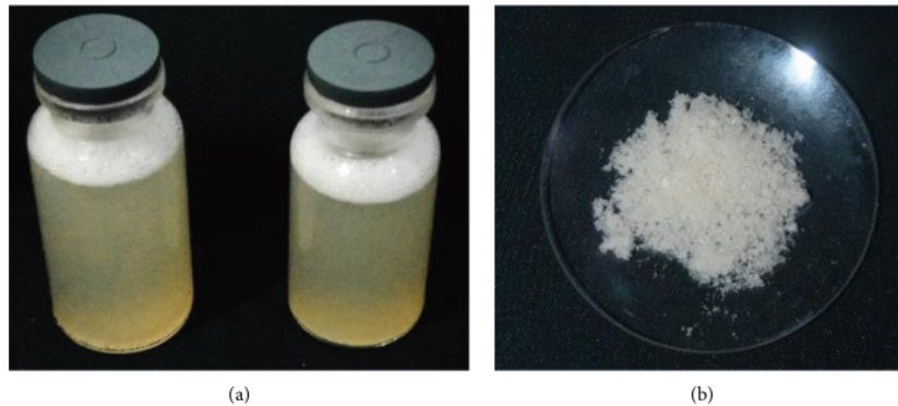
FIGURE 1: The appearance of hydrogels (a) before drying and (b) after the drying process.
